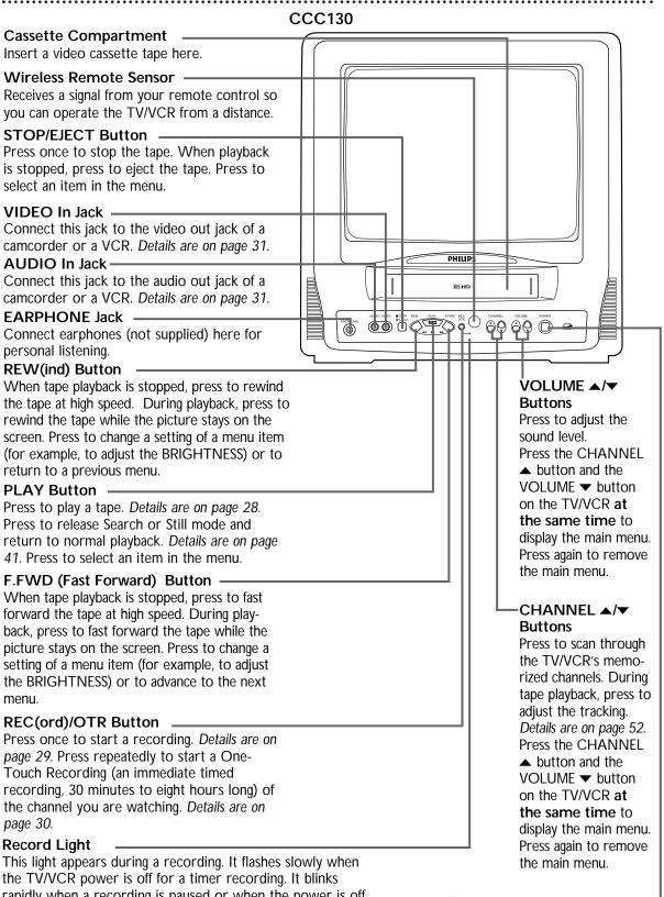
the TV/VCR power is off for a timer recording. It blinks rapidly when a recording is paused or when the power is off for a timer recording, but there is no tape in the TV/VCR. It will blink rapidly two minutes before a timer recording is set to begin if the TV/VCR power is on.
